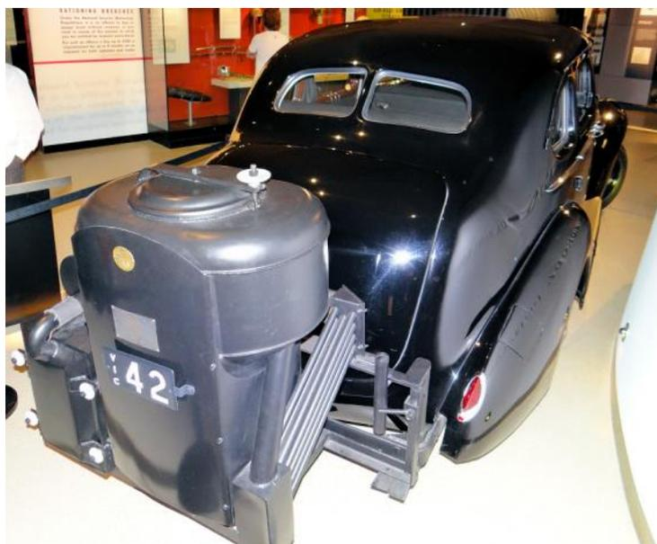
*WW2 Charcoal Gas Produce In this instance fitted to a Studebaker*
