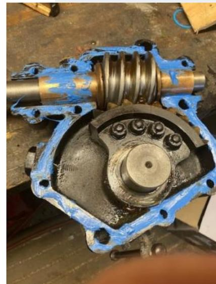
*Restored bus steering box ready for re-installation*
