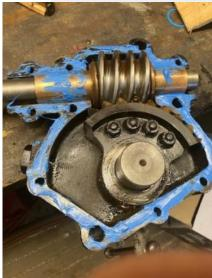
Restored bus steering box ready for re-installation
