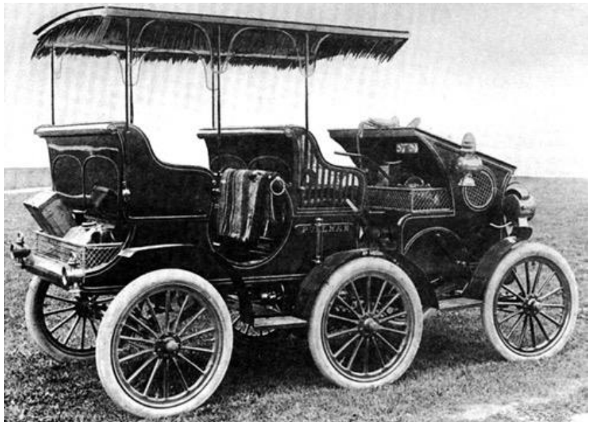
There were Pullman cars on trains but this was the Pullman, a 6-wheeled car built in York, Pennsylvania. The middle wheels did the driving and the front and rears did the steering
