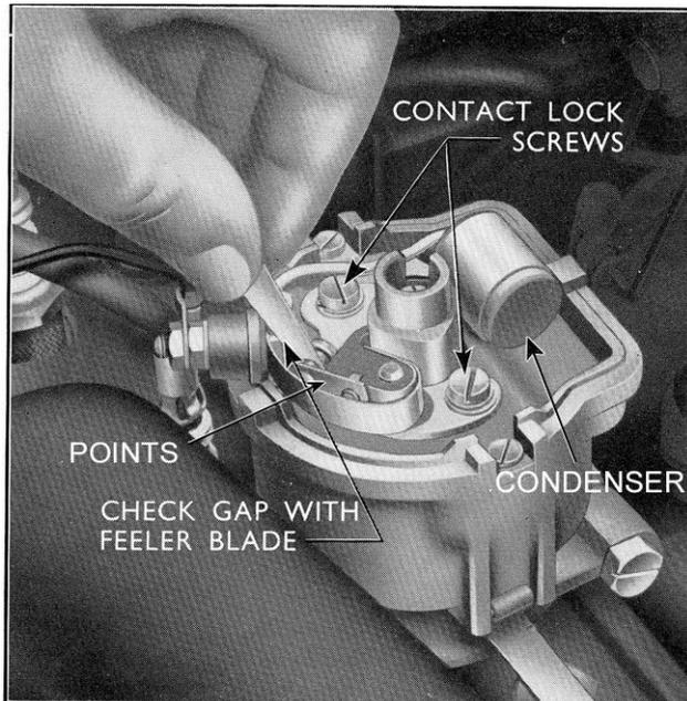
*Inside the distributor, from the workshop manual. The points gap is checked with a feeler blade; 0.015" is the one. The points should be on the heel of the cam, as shown, and so open at their widest, and there should be a slight resistance to moving the blade – a 'magnetic grip', as it is termed. When the engine is turned so that there is no contact between the points' fibre heel and the cam, the points must be fully closed.*
