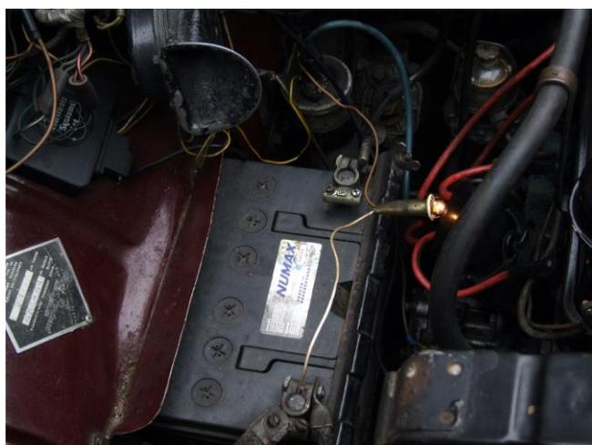
*A simple test lamp made from two lengths of wire and a bulb and holder. Small crocodile clips on the ends of the wires would improve it. It is here connected between the live LT side of the coil and the earth post of the battery. The ignition is on, so the lamp is correctly lit up.*
