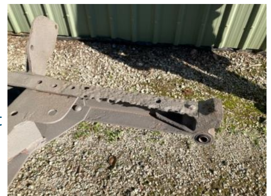
BSA Chassis stripped and rust-proofed. Front members needing repair are shown in the shots below
