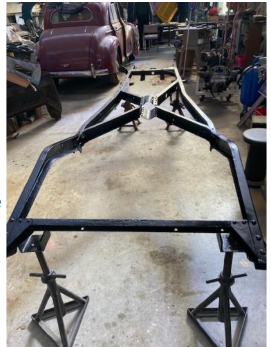
BSA Chassis stripped and rust-proofed. Front members needing repair are shown in the shots below
