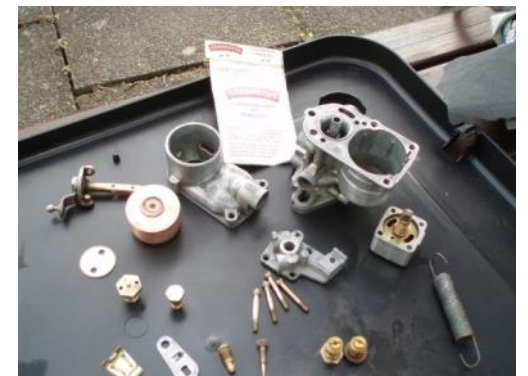
Solex Carb, stripped. Cleaned and reassembled
