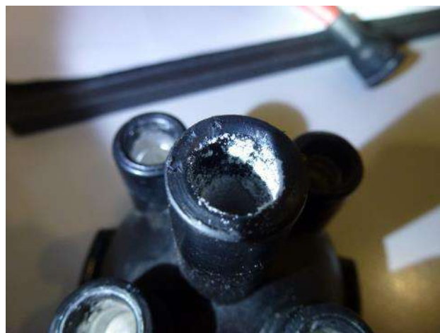
Distributor cap erosion
