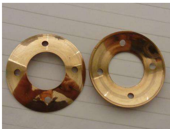
MGB differential thrust washers
