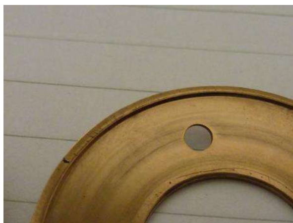
These should be flat at 35 thou’ thick. The worn lip was 10 thou and overall thickness was down to just 20 thou.
