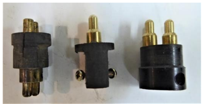
The original sprung terminal with the replacement on the right and the adapted one in the middle.
