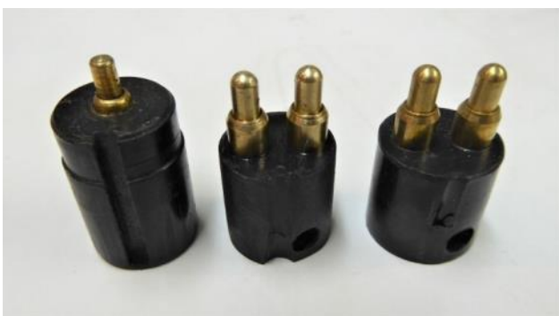
The original sprung terminal with the replacement on the right and the adapted one in the middle.
