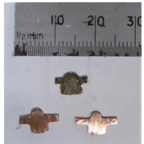
Right: Shaped washers fashioned from copper strip.
