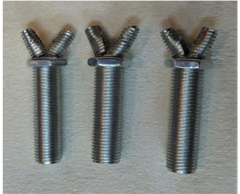
Special bolts made from threaded tube.
