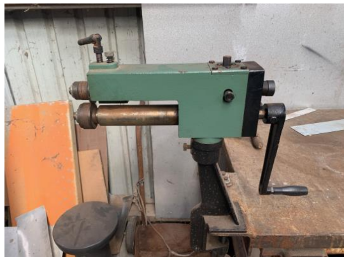
A 'Jenny' otherwise known as a 'Bead Roller'. Does anyone know why its called a Jenny?
