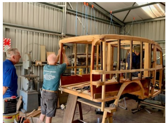
It's all down to mathematics as John Ellis starts the cladding around the rear corners of the BSA load space.
