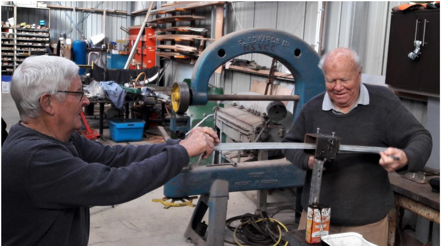
Necessity is the mother of invention: Neville and Peter wheel out a repair panel using Neville's home made roller.
