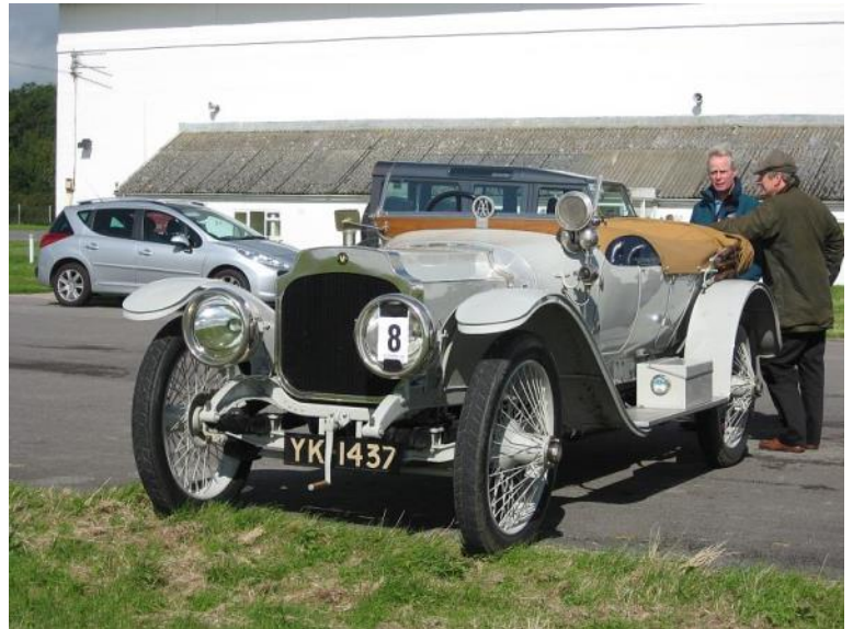
1912 Vauxhall A12, Four cylinders, 95 x 120mm, 3,418 c.c.
