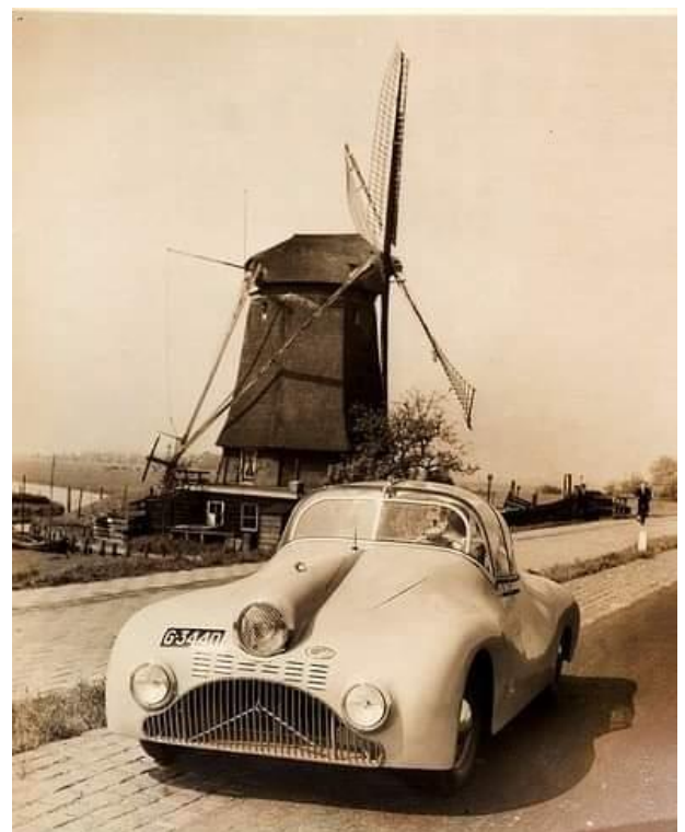
1948 Gatso Roadster. Holland's first postwar car. Plastic Roof and Powered by Ford V8 lump
