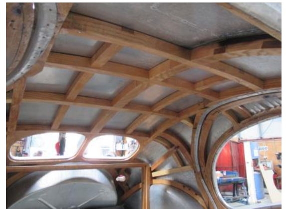
Bugatti roof framing.
