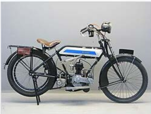
1920 Coventry-Eagle with 2.75 hp JAP four-stroke engine
