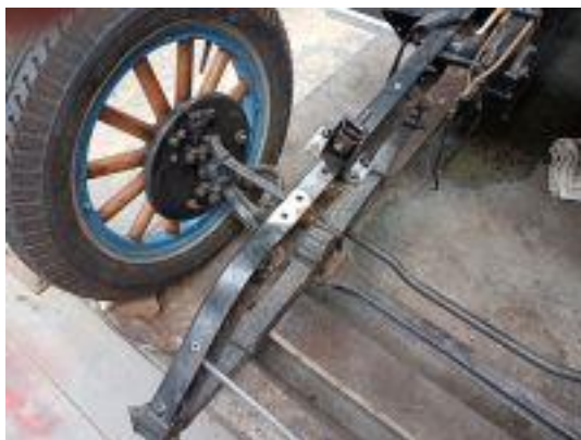
Engine out in order to remove pitted cross member. New item being fabricated now.
