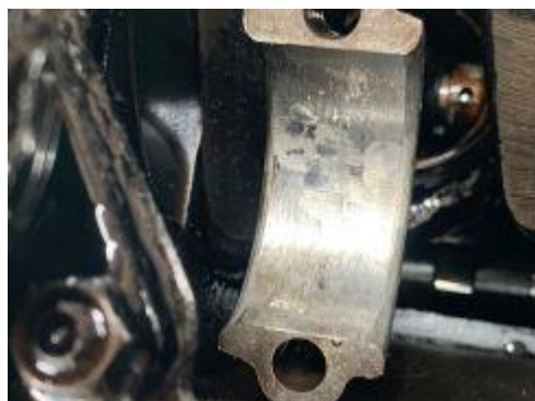
Conrod showing babbitt bearing totally disintegrated, Tony not happy
